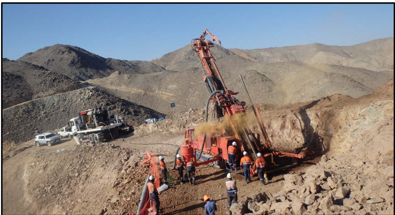
Figure 2: Capital Drilling's rig 256 collaring RC hole ROP-001 at Rodruin
