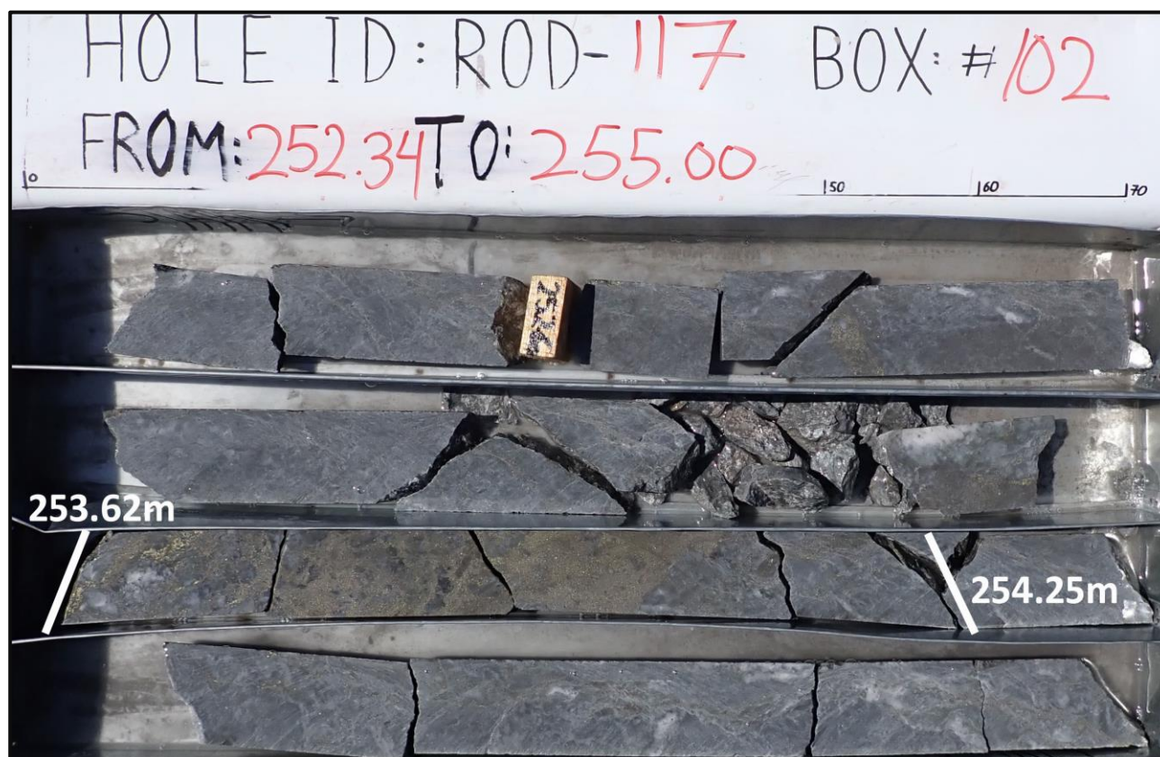
Figure 3: Cut HQ3 sized drill core from hole ROD-117, showing the very high grade sulphide-rich interval between 253.62m – 254.25m
