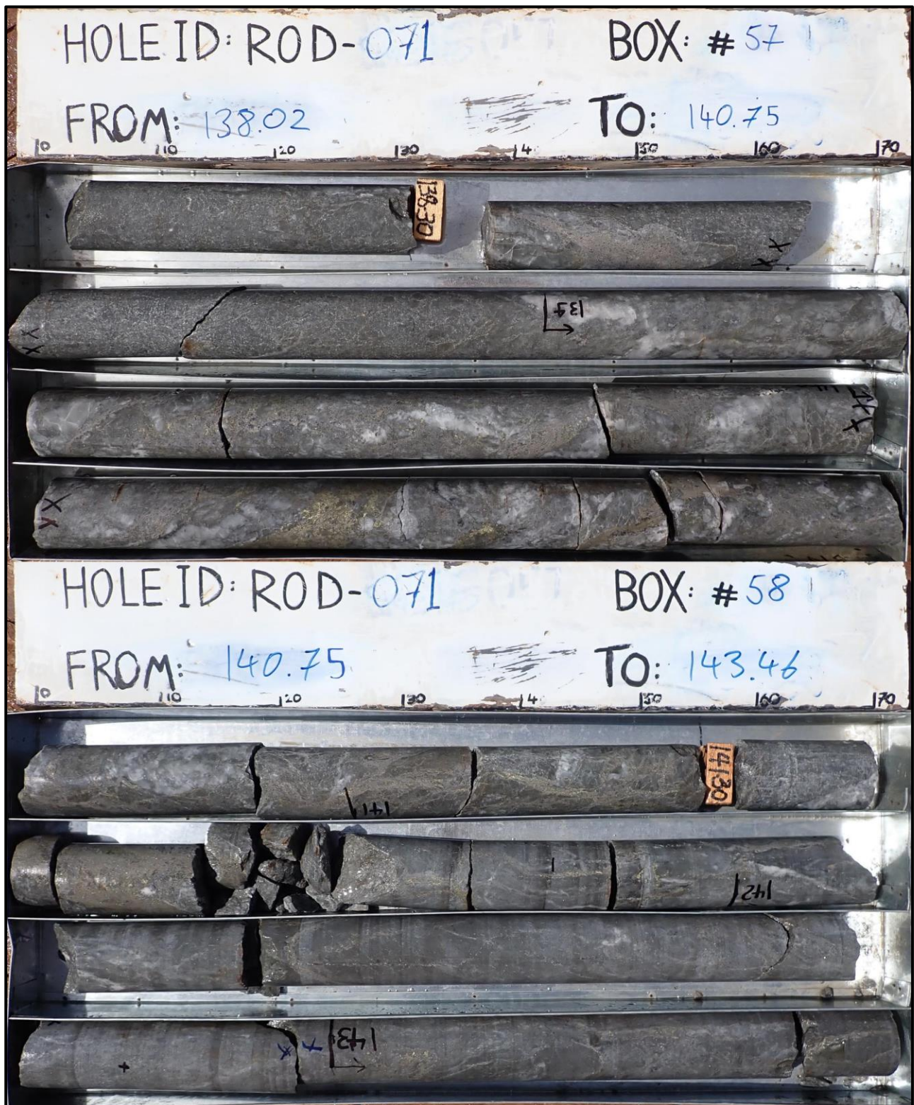
Figure 4: ROD-071 drill core from 138.02-143.46m (note the chalcopyrite at approximately 140.3m, and the network veins of pale grey sphalerite, prominent at about 138.4 and 141.0m)
