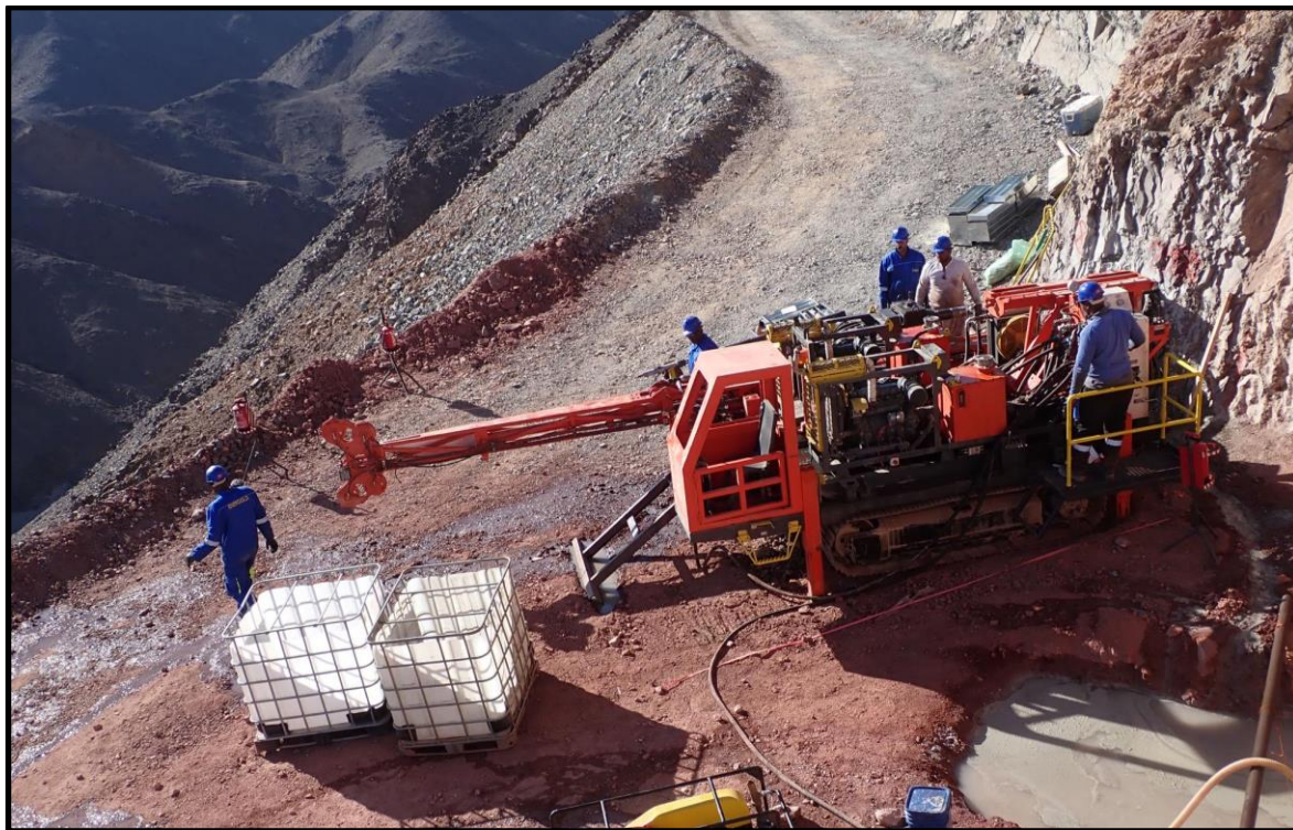
Figure 2: Energold's ID500-G rig drilling on the first hole of the new programme, ROD-051
