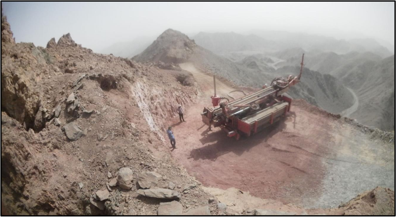
Figure 2: Fisheye view looking to the south, of the drill rig setting up at the Spiral Pit zone (note sharp fault contact in pad between red mineralised gossan and grey-green unmineralised metasediments)
