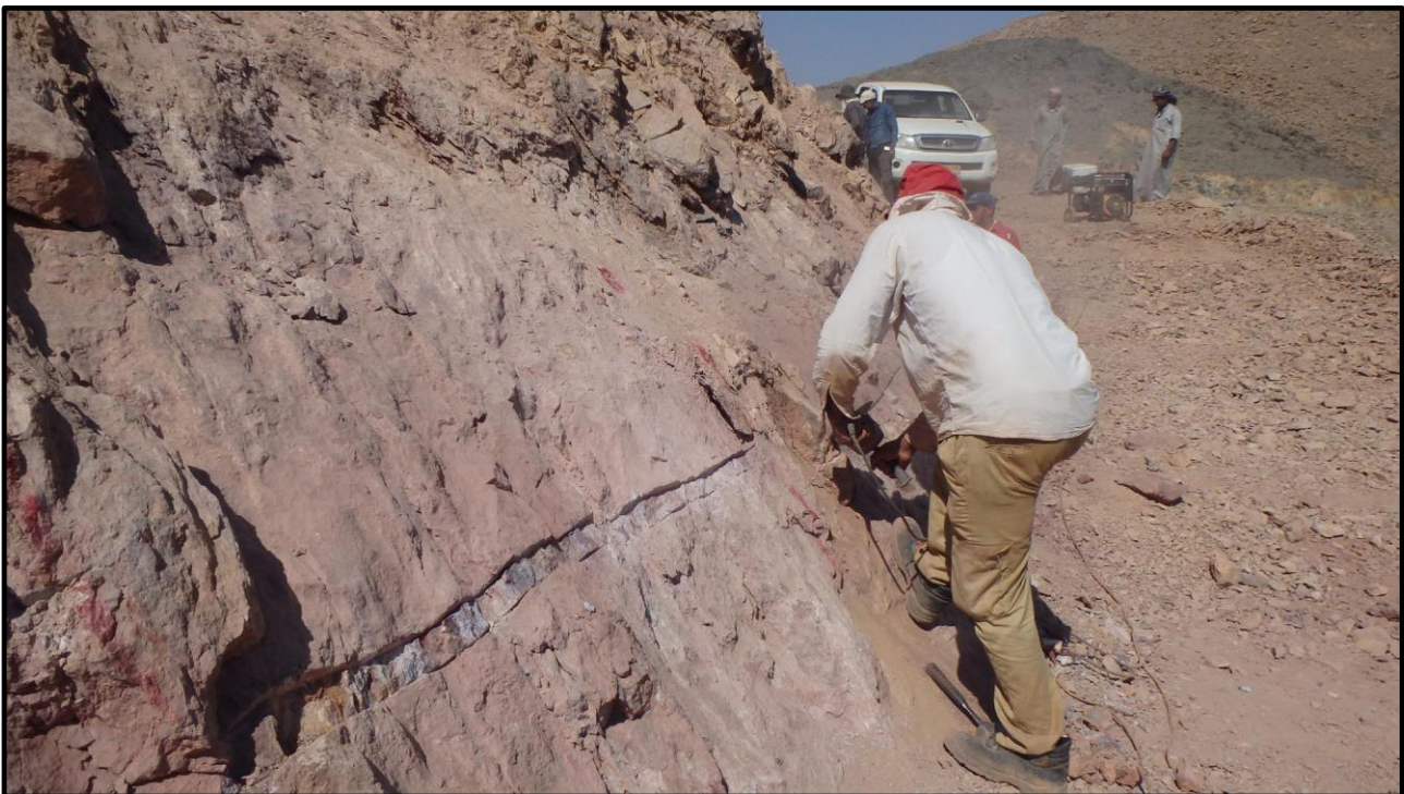
Figure 4: Channel sampling altered and well mineralised slates in the ROC-005 profile at Aladdin's Hill
