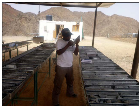
Figure 10-6 Logging diamond drill core at the core farm
